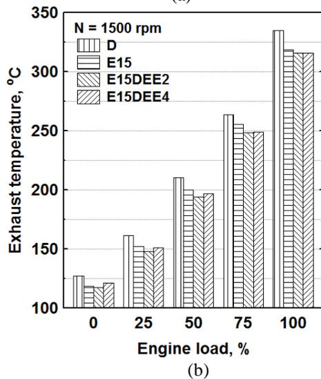
Fig. 5. Air excess coefficient and exhaust gas temperature for the tested fuels
