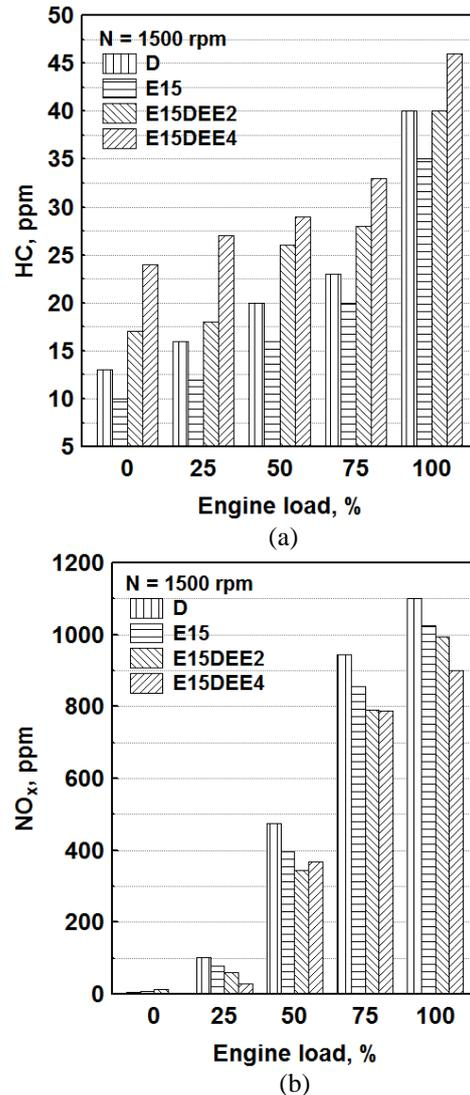
Fig. 9. HC and NO<sub>x</sub> emissions for the tested fuels
