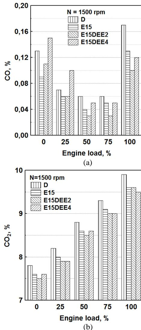
Fig. 8. CO and CO<sub>2</sub> emissions for tested fuels
