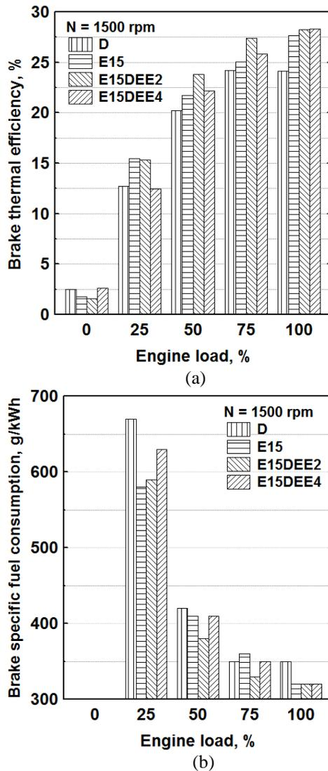
Fig. 7. Brake thermal efficiency and specific fuel consumption for the tested fuels
