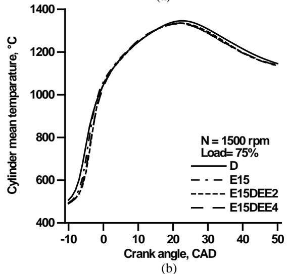
Fig. 4. Cylinder pressure and cylinder mean temperature for the tested fuels
