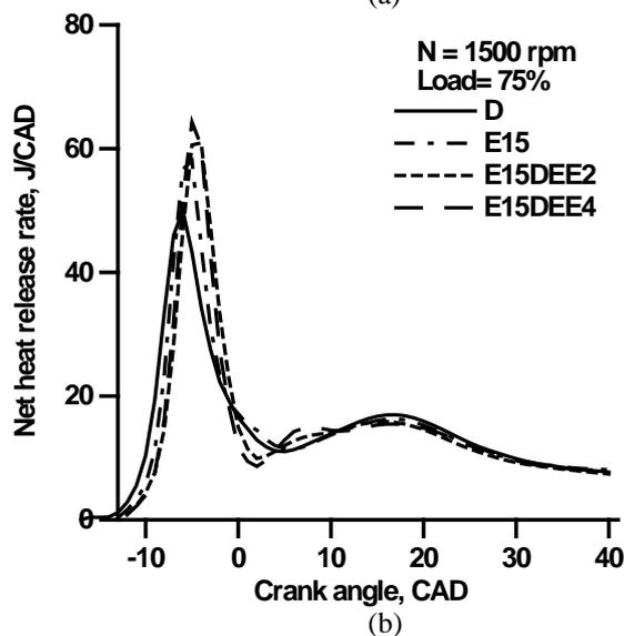
Fig. 3. Burnt mass fraction and heat release rate for the tested fuels
