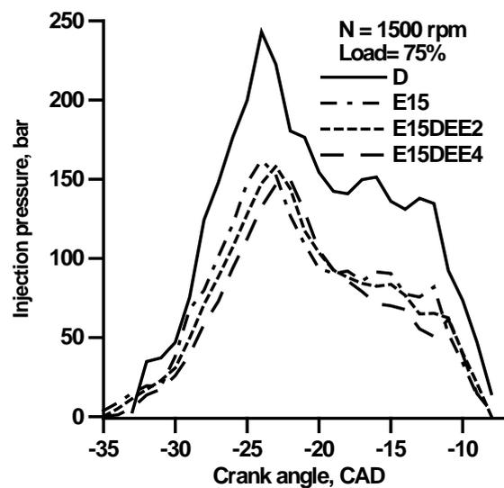
Fig. 2. The injection pressure for the tested fuels
