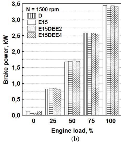
Fig. 6. Brake torque and power for the tested fuels
