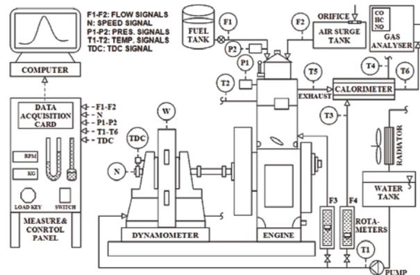
Fig. 1. The schematic layout of the test setup
