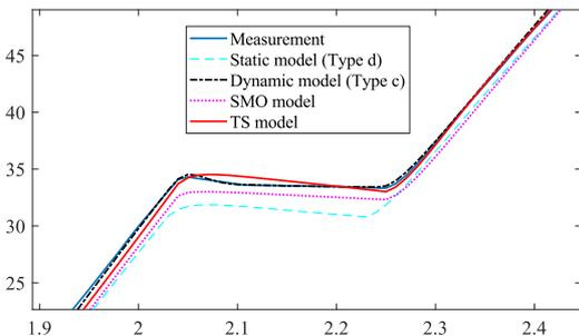
Fig. 5 Measurement and model prediction with static models for range  $[1.9 \text{ s}; 2.4 \text{ s}]$
