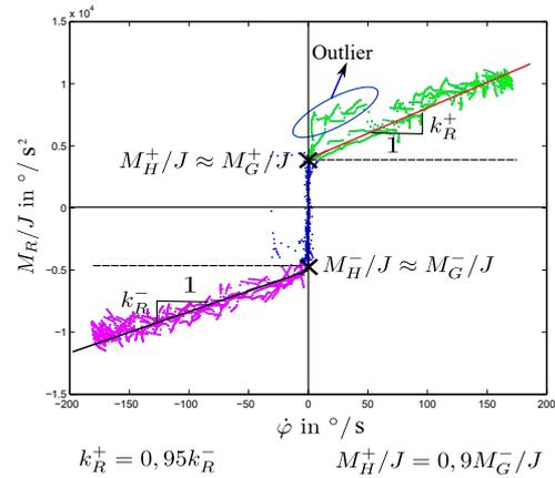
Fig. 3 Velocity-friction data map with straight approximation lines and estimated parameters of the friction model
