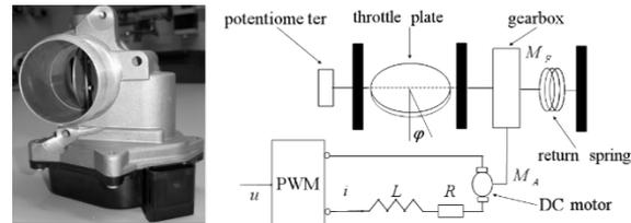
Fig. 1 Throttle and its technology scheme
