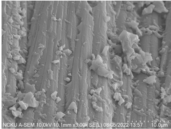
Fig. 24. The fractography of the material added with 0.4wt% aerogel (3000x SEM).
