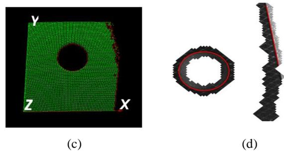
**Figure 6.** An example of the 3D edge detector using Laplacian. (a) original image; (b) point cloud of scene ; (c) results of the 3D edge detector using Laplacian; (d) result of mapping 3D edge points to 2D image.
