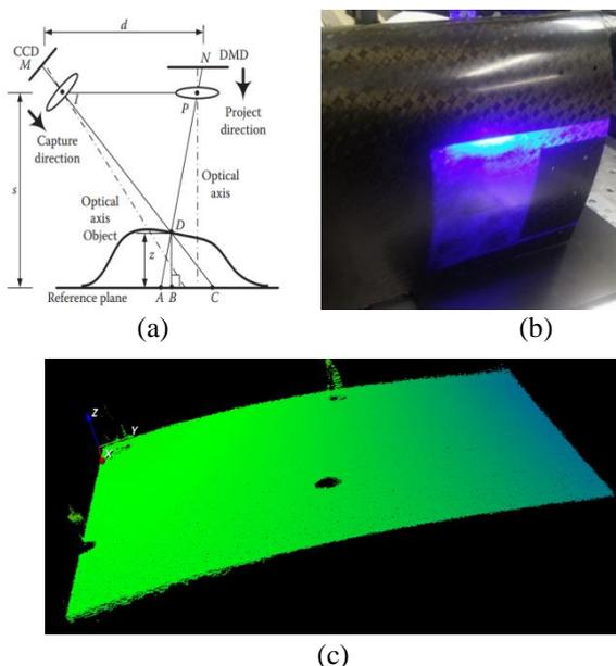
**Figure 7.** (a) optical configuration in 3D measurement; (b) actual measurement of the aerospace composite part; (c) 3D point cloud being reconstructed.
