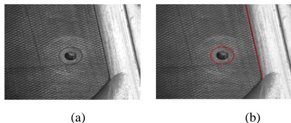
**Figure 1.** An example of feature detection. (a) the original image; (b) expected result.
