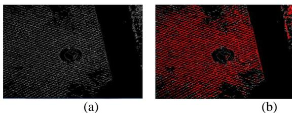
**Figure 2.** Example of image segmentation result using conventional image processing techniques: (a) using Canny edge detection; (b) using Hough line transform.
