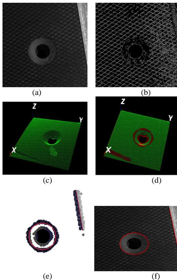
**Figure 8.** (a) original image; (b) result of Canny edge detection; (c) point cloud of ROI ; (d) result of the 3D edge detector; (e) result of 2D feature detectors performed on the extracted edge regions; (f) the final result of developed method.
