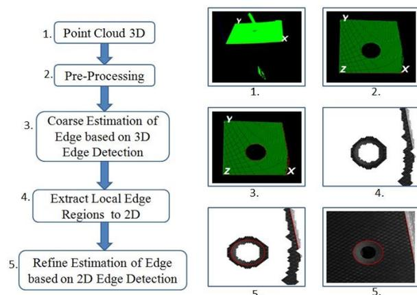
**Figure 4.** Flowchart of proposed multi-dimensional image fusion algorithm for feature detection.
