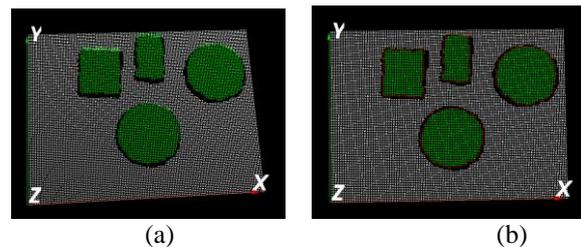
**Figure 3.** The outputs of 3D image feature detection: (a) point cloud being detected by 3D vision technique; (b) missing object edges being marked Red due to optical diffraction disturbance.
