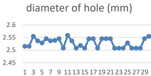
**Figure 9.** 30-times diameter measurement result of machined hole.
