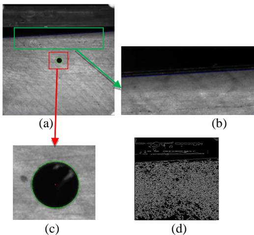
**Figure 10.** (a) feature detection of a shiny surface; (b) zoom of edge line; (c) zoom of circle; (d) result of Canny edge detection.
