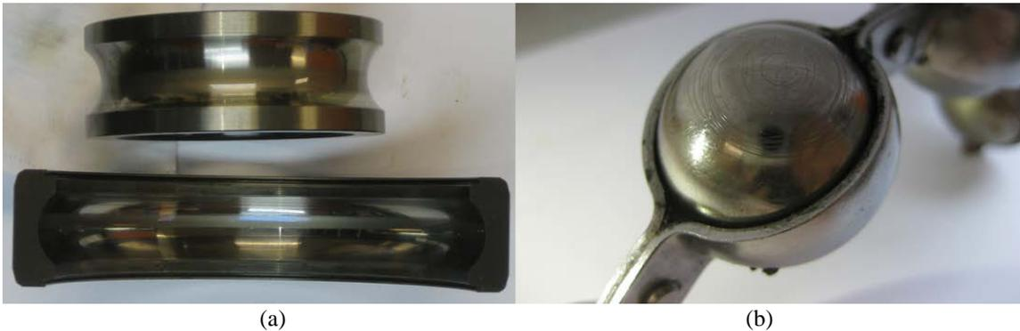
Fig. 9. Motor sample 5 drive-end bearing defects (a) bearing inner and outer ring, (b) ball bearing
