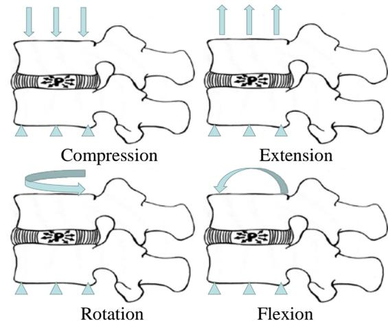
Fig. 4. Boundary condition and loads in the simulation
