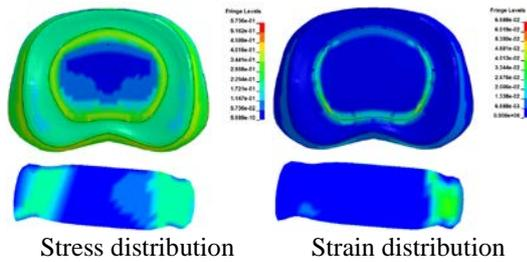
Fig. 7. Comparison of stress and strain distribution under compression in disc (80 ms)
