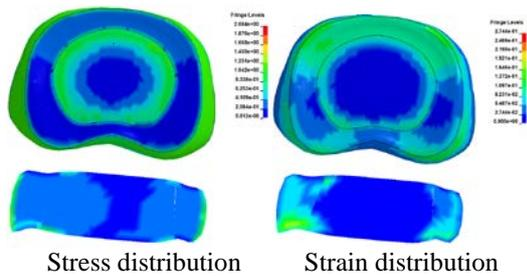
Fig. 8. Comparison of stress and strain distribution under rotation condition in disc (40 ms)
