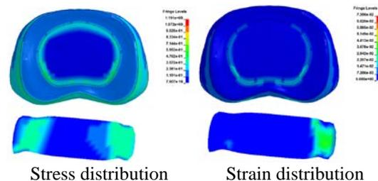
Fig. 6. Comparison of stress and strain distribution under extension in disc (80 ms)
