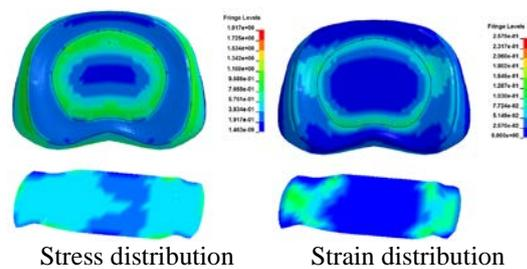
Fig. 9. Comparison of stress and strain distribution under flexion condition in disc (40 ms)
