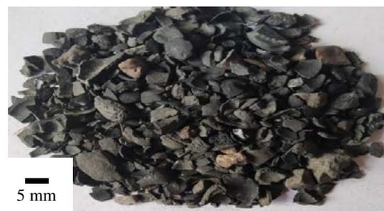
Fig. 4. Biochar generated after the pyrolysis of oil palm kernel shells (source:Yuan Da Technology Co., Ltd.)
