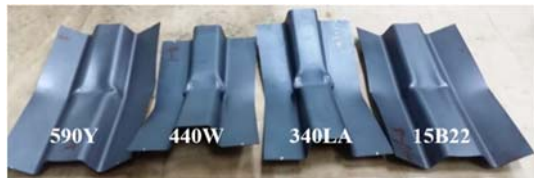
Fig. 9. Experimental results for the single property blank with opening groove
