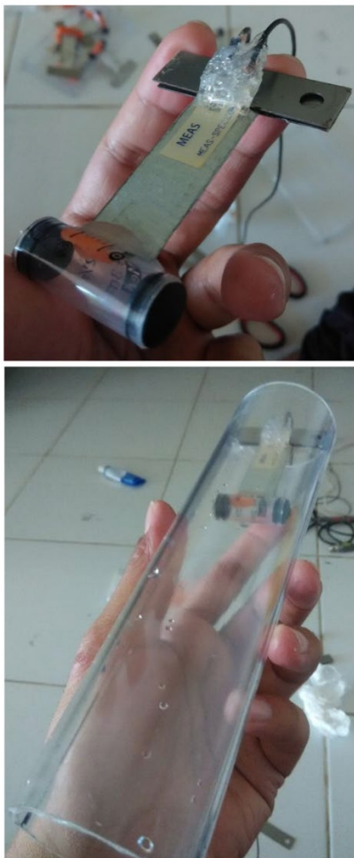
Fig. 4. VIV Apparatus Inside Converter Pipe
