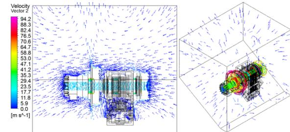
Fig. 5. Distribution of flow fields of the lathe spindle system (base). (a): interior, cross-section along the center of the spindle (b) exterior of the spindle system.
