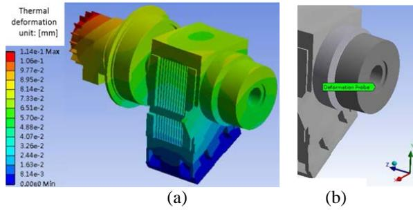
Fig. 6. Thermal deformation (a) and the probing position of the spindle system.
