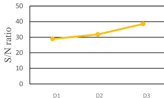
**Fig. 10.** The effect of coolant flow speed based on the S/N ratio.
