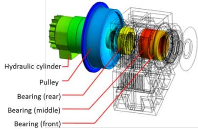
Fig. 3. Schematic diagram of heat source distribution in the spindle system.
