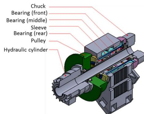
Fig. 1. Schematic diagram of the lathe spindle system in current study.
