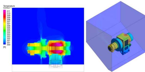
Fig. 4. Temperature field distribution inside the lathe spindle system (base). (a): interior, cross-section along the center of the spindle (b) exterior of the spindle system.
