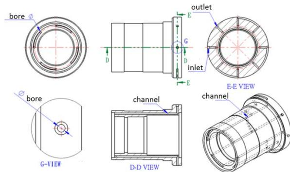
Fig. 2. Schematic diagram of the spindle sleeve cooling channel design
