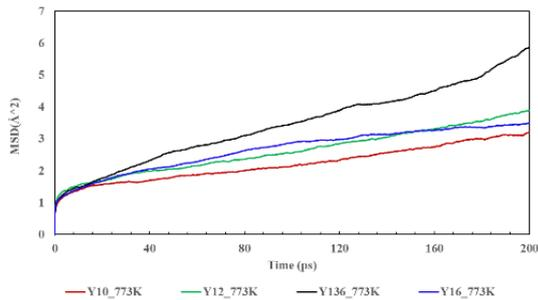
Figure 3. Comparing the Hydrogen MSD with different doping ratio of Y
