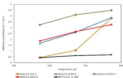
Figure 6. Comparing the diffusion coefficient of BZY with temperature effect and doping effect
