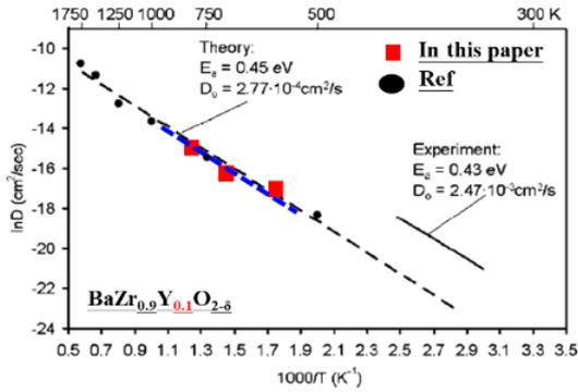
Figure 2. Comparing the diffusion coefficient of BZY between previous work and this paper
