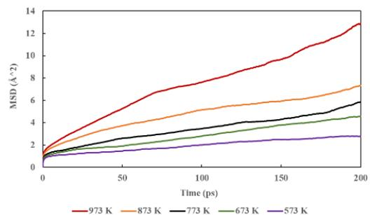
Figure 4. Comparing the Hydrogen MSD with different working temperature
