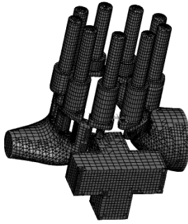
Fig. 4. Mesh grid model of a piston pump.
