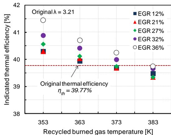
Fig. 12. Indicated thermal efficiency at different EGR ratios and  $T_{EGR}$  (original  $\lambda = 3.21$ ).
