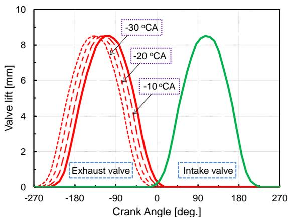
Fig. 3. The valve lift profiles for internal EGR studies.
