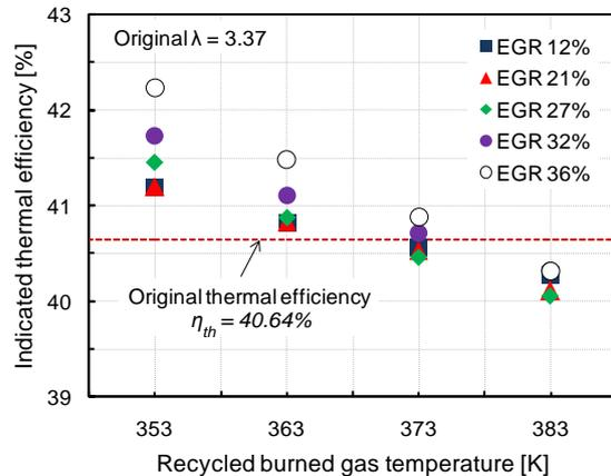
Fig. 11. Indicated thermal efficiency at different EGR ratios and  $T_{EGR}$  (original  $\lambda = 3.37$ ).
