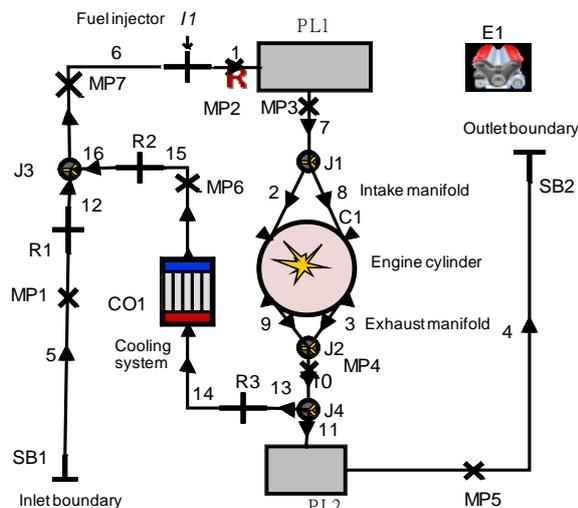
Fig. 1. AVL-5402 engine model on AVL BOOST.
