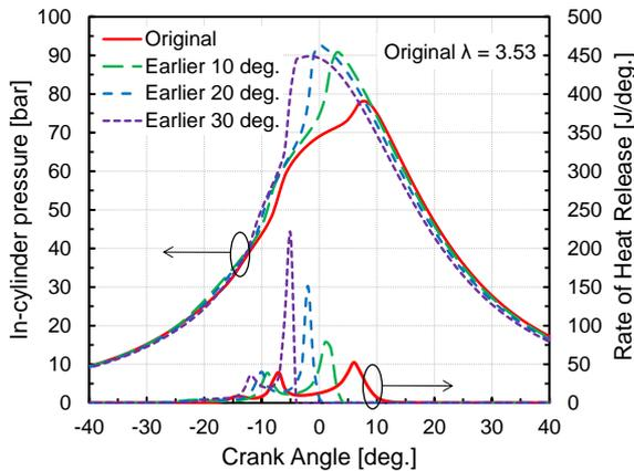
Fig. 5. Pressure and ROHR profiles at different timing of exhaust valve opening (original  $\lambda = 3.53$ ).
