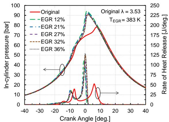
Fig. 7. Pressure and ROHR profiles at different EGR ratios and  $T_{EGR} = 383K$  (original  $\lambda = 3.53$ ).
