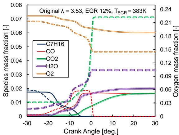
Fig. 8. Species mass fraction at original  $\lambda = 3.53$  (solid line); EGR 12% and  $T_{EGR} = 383K$  (dash line).
