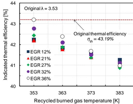
Fig. 10. Indicated thermal efficiency at different EGR ratios and  $T_{EGR}$  (original  $\lambda = 3.53$ ).
