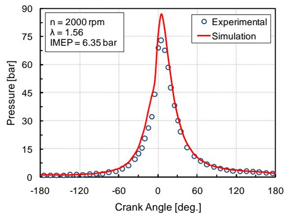
Fig. 2. Pressure curves from experiment and simulation data under CI mode.
