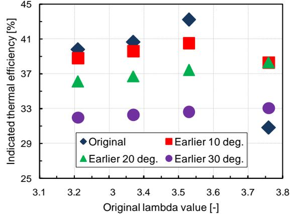
Fig. 6. Indicated thermal efficiency at different opening time of exhaust valve and original  $\lambda$ .
