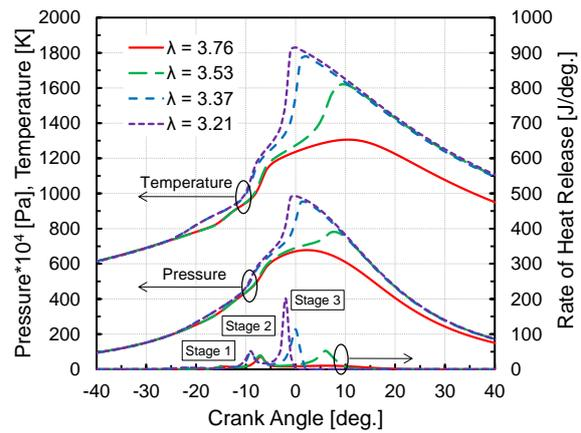
Fig. 4. The pressure, temperature and ROHR profiles at different value of lambda.
