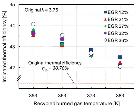
Fig. 9. Indicated thermal efficiency at different EGR ratios and  $T_{EGR}$  (original  $\lambda = 3.76$ ).
