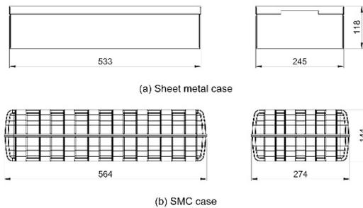
Fig. 2. Dimension of the (a) Sheet metal case and (b) SMC case
