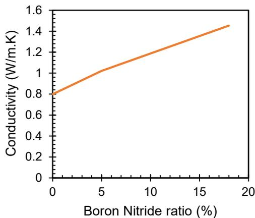
Fig. 3. Thermal conductivity of SMC
