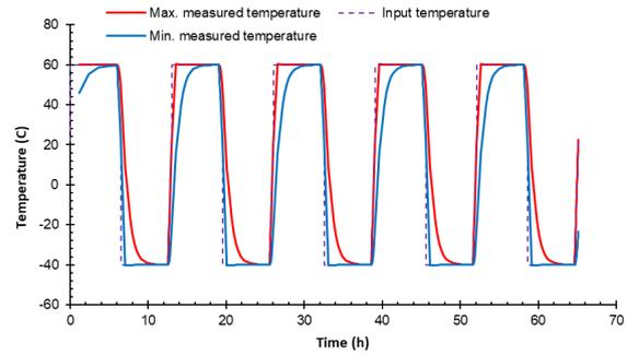
Fig. 11. Comparison Between Input and Measured Temperature on Sheet Metal Case
