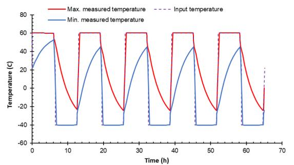
Fig. 12. Comparison Between Input and Measured Temperature on SMC Case
