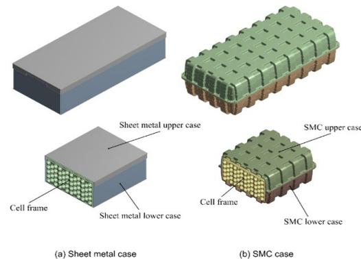
Fig. 1. Components of the (a) Sheet metal case and (b) SMC case
