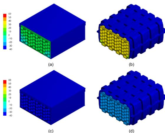
Fig. 15. Temperature distribution in III (a-b) and IV (c-d) steps of thermal cyclic test on Sheet metal case and SMC case
