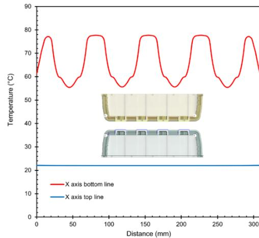
Fig. 9. Profile of temperature distribution along X axis top and bottom line on SMC case
