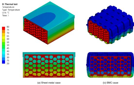
Fig. 6. Thermal distribution on (a) Sheet metal case and (b) SMC case
