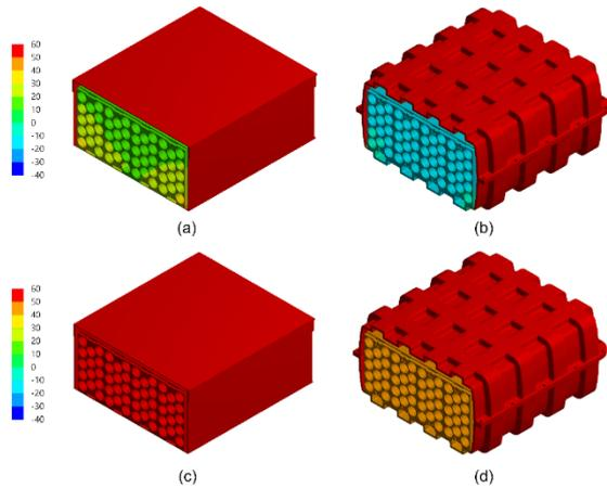
Fig. 14. Temperature distribution in I (a-b) and II (c-d) steps of thermal cyclic test on Sheet metal case and SMC case
