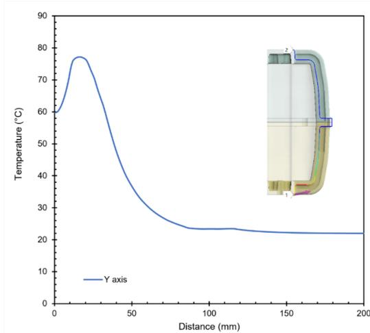
Fig. 10. Profile of temperature distribution along Y axis line on SMC case
