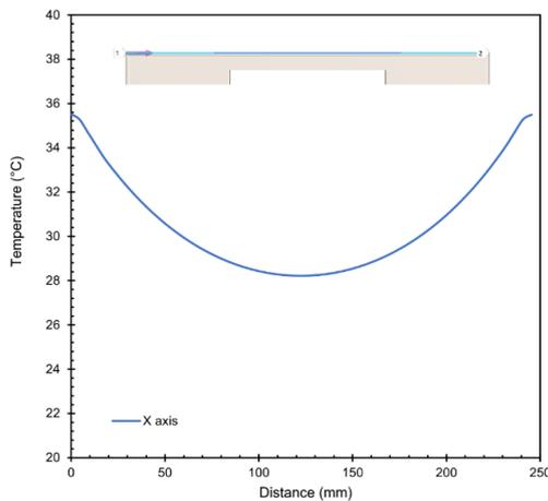
Fig. 7. Profile of temperature distribution along X axis line on top cover of Sheet metal case
