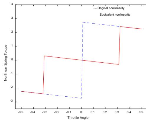
Fig. 13. Equivalent nonlinearity  $\bar{n}$  (solid line) expressed in Eq. (17). Original nonlinearity  $T_s$  (dashed line) expressed in Eq. (3).
