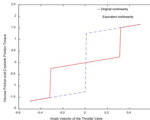
Fig. 14. Equivalent nonlinearity  $\bar{n}$  (solid line) expressed in Eq. (17). Original nonlinearity  $T_f$  (dashed line) expressed in Eq. (4).
