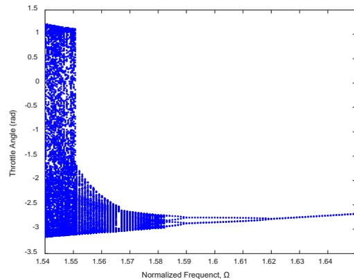
Fig. 2. Bifurcation diagram of throttle valve angle vs.  $\Omega$ .
