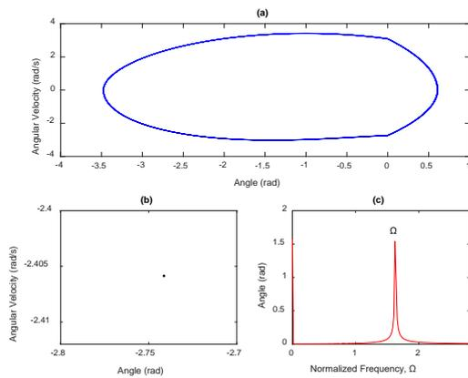
Fig. 3. Period-1 orbit of numerical simulation results for  $\Omega = 1.63$ :
