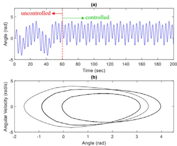
Fig. 15. Square-wave dither signal was injected to control chaotic motion of electronic throttle system for  $W = 0.315$  and  $\Omega = 1.542$ : (a) time responses of controlled system; (b) phase portrait of controlled system. Square dither signal was introduced after 60 s.
