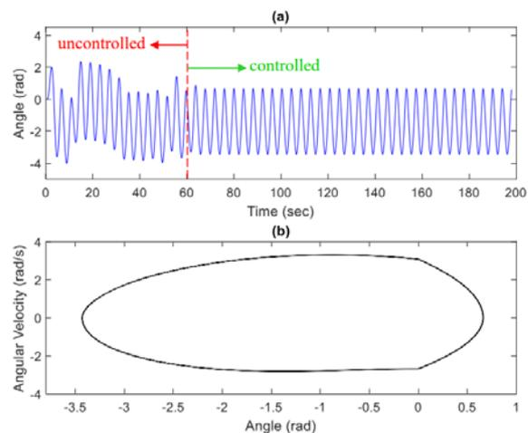
Fig. 10. Transformation of chaotic motion into period-1 orbit for  $K = -0.2$  and  $\Omega = 1.542$ : (a) time responses of controlled system; (b) phase portrait of controlled system. State feedback control signal was introduced after 60 s.
