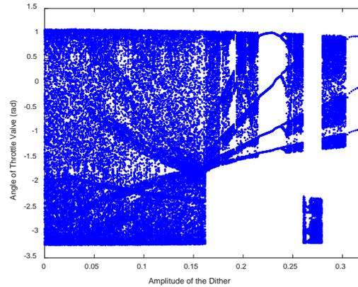
Fig. 12. Bifurcation diagram of throttle valve angle against  $W$  for electronic throttle system with square-wave dither, where  $W$  represents dither amplitude.
