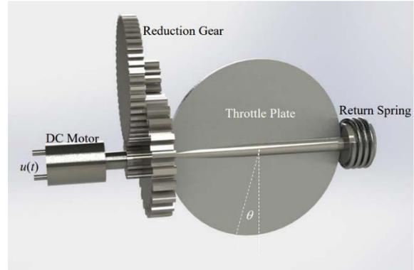
Fig. 1. Schematic of electronic throttle system.
