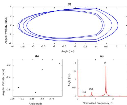
Fig. 5. Period-4 orbit of numerical simulation results  $\Omega = 1.584$ :
