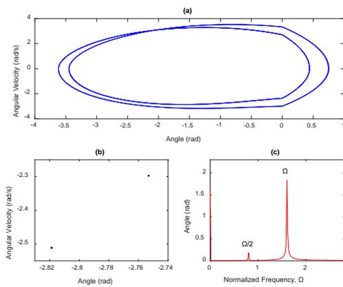
Fig. 4. Period-2 orbit of numerical simulation results for  $\Omega = 1.61$ :
