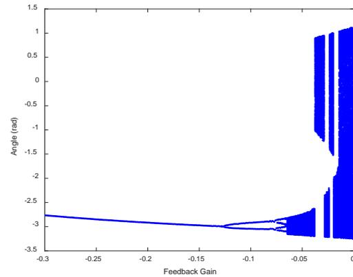
Fig. 9. Bifurcation diagram of throttle valve angle against  $K$  for electronic throttle system with state feedback control, where  $K$  indicates feedback gain.
