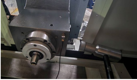
Fig. 9. Schematic for modal testing.
