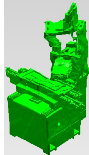
Fig. 12. Modal testing, mode 2:146.0 Hz.
