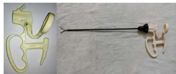
Figure 4. Modified laparoscopic forceps handle
