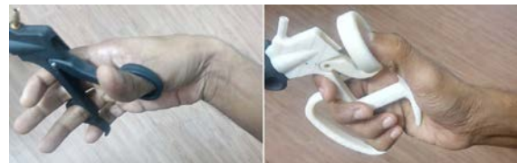
Figure 7. Wrist posture when using existing (left) and modified (right) laparoscopic forceps handles
