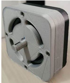
Figure 10. 3D Printed image of Model 10 Z58-Z60 20^\circ harmonic Reducer
