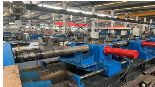
Fig.16 Horizontal bench test of 178mm vertical drilling tool
