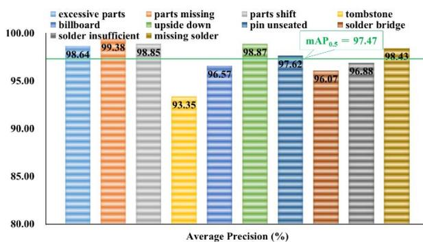
Figure 5. Average precision of PCBA defect classification based on multi-scale training and learning rate decay scheme.
