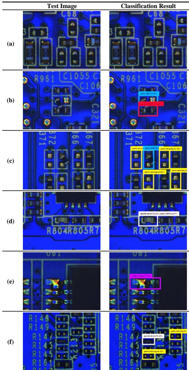
Figure 6. Illustration of some test images: (a) An image without defects; (b) An image has two defects; (c) An image has several defects; (d) An image has two defects at the same position; (e) Defect “pin unseated” is misjudged as “solder bridge”; (f) An image has three defects, one of which is that the “billboard” is misjudged as “upside down”.
