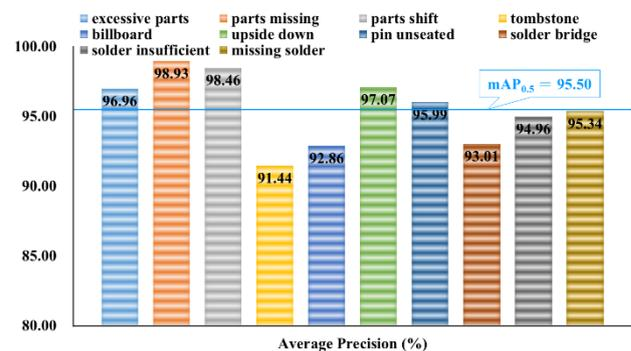
Figure 3. Average precision of PCBA defect classification using multi-scale method.
