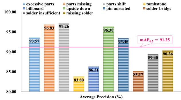
Figure 2. Preliminary training precision of PCBA defect classification using YOLOv3.
