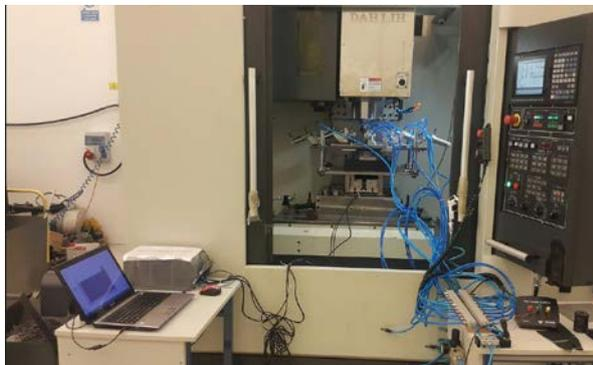
Fig. 13. Using of force measuring system on CNC machining center.
