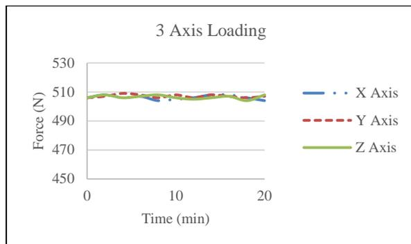
Fig. 12. 3 axis load application test results for 20 min.
