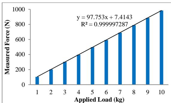
Fig. 9. Z-axis measurement values (kg-Newton)
