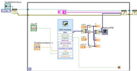
Fig. 5. Force measurement system block diagram.
