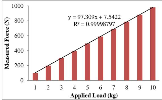
Fig. 7. X-axis measurement values (kg-Newton).
