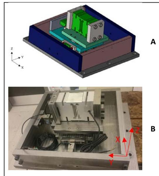
Fig. 2. Force measurement system. A: Design installation, B: Manufactured
