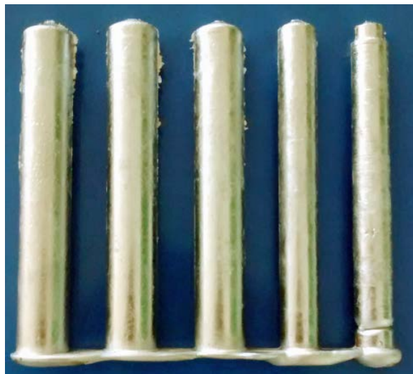
Fig.2. Cast Specimen of ZA-27 nanocomposite
