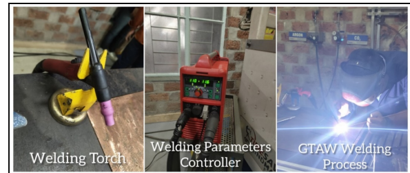
Fig. 3. GTAW Welding Setup.
