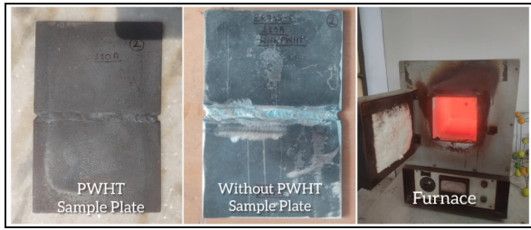
Fig. 4. Post Weld Heat Treatment (PWHT).
