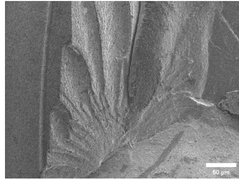
Fig. 9(a). SEM fractographs of specimens deformed at 25°C under strain rates of 4000 s -1 .
