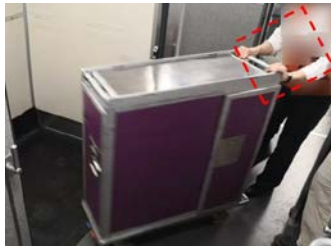
Fig. 5. Static electricity measurement positions on the service cart
