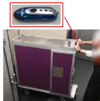
Fig. 11. The electrostatics reduction equipment installed on the service cart
