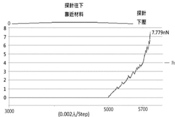
Fig. 2. Simulated down force of molecular statics nanocutting model with probe tip radius 2nm, down-press depth 0.14nm, and  $D$  value 3.032
