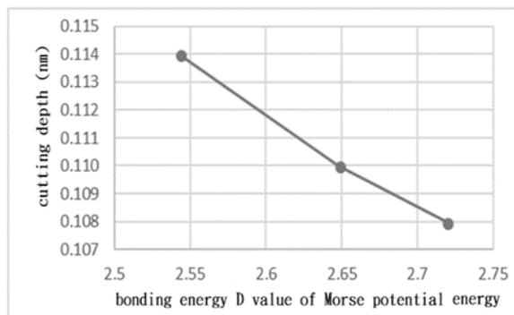
Fig. 6. Relationship diagram between the bonding energy D value of Morse potential energy and the cutting depth
