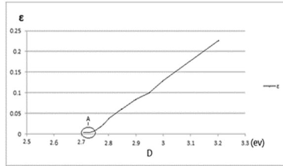
Fig. 3. Relationship diagram between the bonding energy D value of Morse potential energy of the chemical reaction layer of the single-crystal silicon substrate dipped in slurry at 30°C and the convergence value  $\epsilon$
