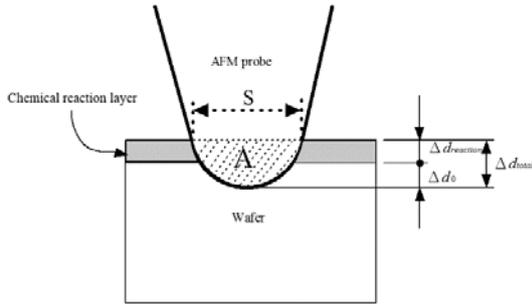
Figure 1 Schematic diagram of chemical reaction layer
