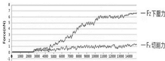
Fig. 5. Stable average down force 6.853nN and stable average cutting force 1.305nN obtained from simulation of molecular statics nanocutting model with D value 2.719ev of the chemical reaction layer of the single-crystal silicon dipped in slurry at 30°C, and with probe tip radius 2nm and cutting depth 0.14nm
