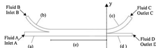
Figure 6 Microfluid system (Cardoso et al., 2018)
