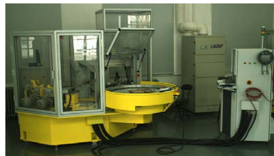
Fig. 5. Intelligent integrated grinding and measuring workcell for blade edges.
