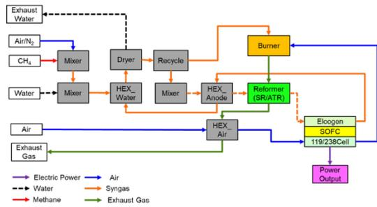
Figure. 1 Schematic diagram of the SOFC system
