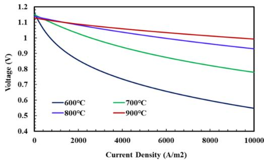
Figure. 3 Polarization curves of the solid oxide fuel cell at different operating temperatures
