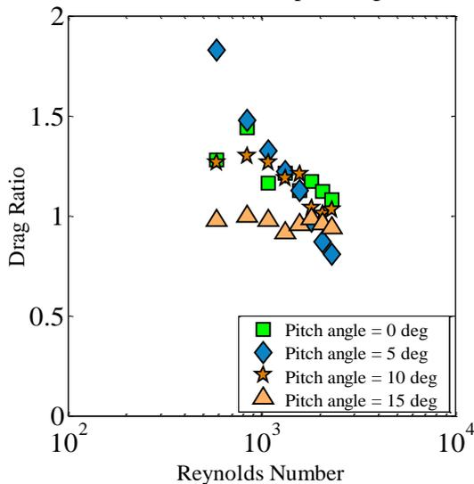
Fig. 8 (b) Drag Ratio ( $D_{TS}$ ) for various pitch angle
