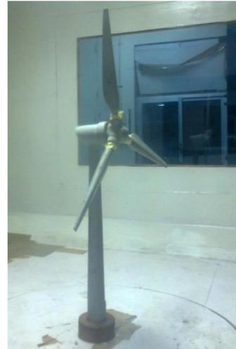
Fig. 1(b) Experimental pressure model in Wind tunnel
