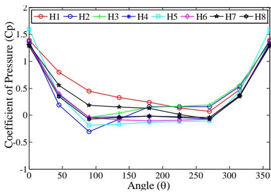
Fig. 6 Maximum Pressure coefficient ( $C_p$  max) on wind turbine tower with rotor blades at Free-stream velocity  $V_\infty = 6.25$  m/s and pitch angle  $\phi = 0^\circ$ .
