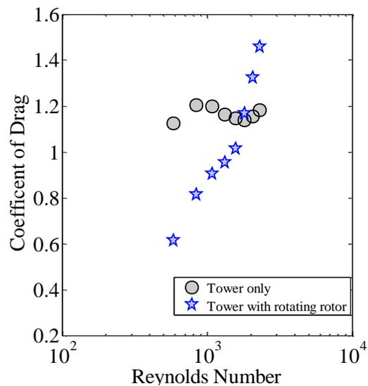
Fig. 7 (a) Coefficient of Drag ( $C_D$ ) calculated for the Tower only and Tower with rotating rotor.
