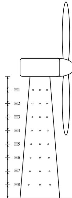
Fig. 2 (a) Schematic of wind turbine model with pressure probes on various heights, Not to scale
