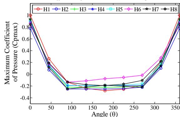
Fig. 4 Mean Pressure coefficient ( $C_p$  mean) on wind turbine tower with rotor blades at free-stream velocity  $V_\infty = 6.25$  m/s and pitch angle  $\phi=0^\circ$ .
