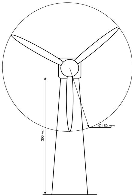
Fig. 2 (b) Schematic and geometric coordinate system of wind turbine model, Not to scale.
