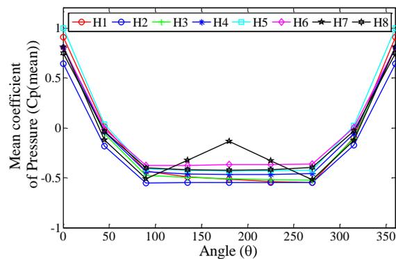
Fig. 3 Mean Pressure coefficient ( $C_p$  mean) on wind turbine tower without the rotor blades at Free-stream velocity  $V_\infty = 6.25$  m/s.
