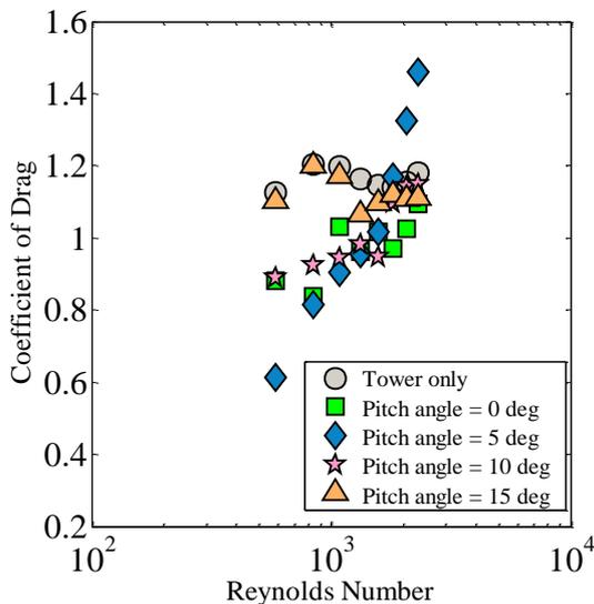
Fig. 8 (a) Coefficient of Drag ( $C_D$ ) with Reynolds number for various pitch angles
