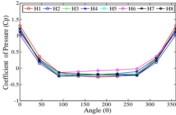
Fig. 5 Maximum Pressure coefficient ( $C_p$  max) on wind turbine tower without the rotor blades at free stream velocity  $V_\infty = 6.25$  m/s.
