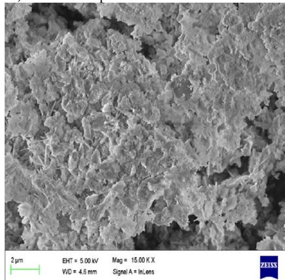
b)SEM of B<sub>4</sub>C particles
