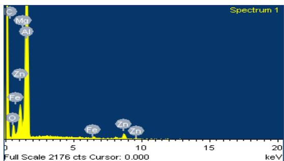
Fig.10(a). SEM and EDX analysis of worn surface for sample A0
