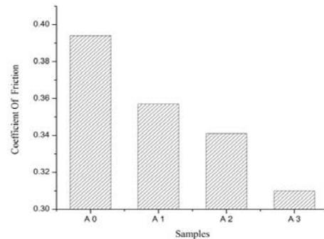
Fig.9. Effects of B<sub>4</sub>C and CDA on coefficient of friction
