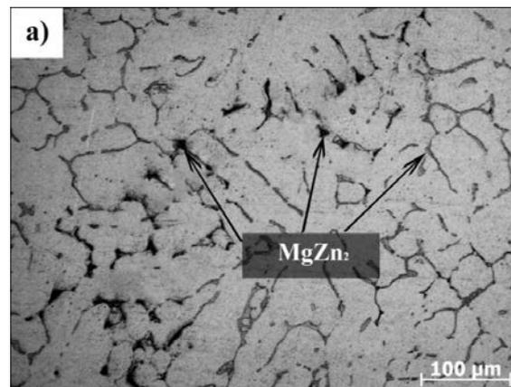
Fig.4 (a). Microstructure for sample A0
