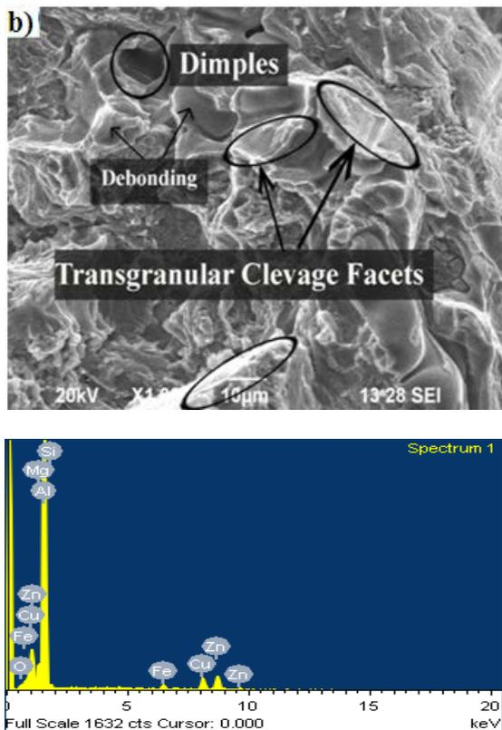
Fig.7(b). SEM and EDX analysis of fractured tensile strength for sample A3
