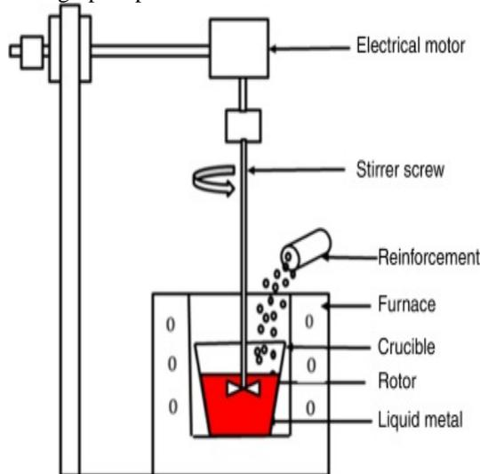
Fig.2. Schematic view of stir casting setup
