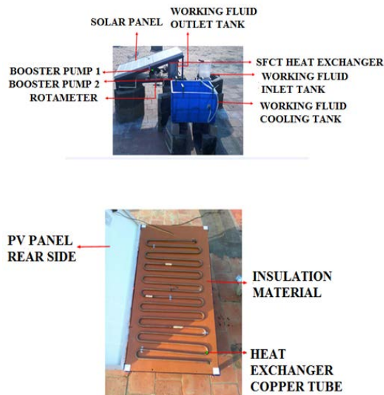
Fig. 2(a) Photographic view of the SPV/T experimental system (b) Serpentine flow copper tube heat exchanger
