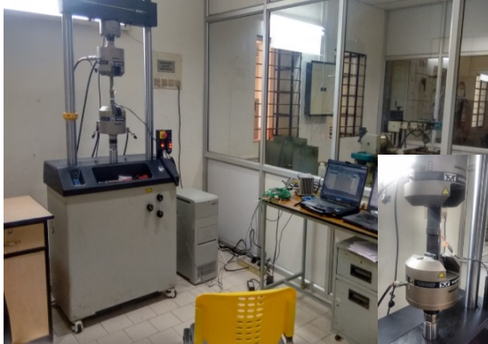
Fig. 5. Fatigue test of backing strip joint.
