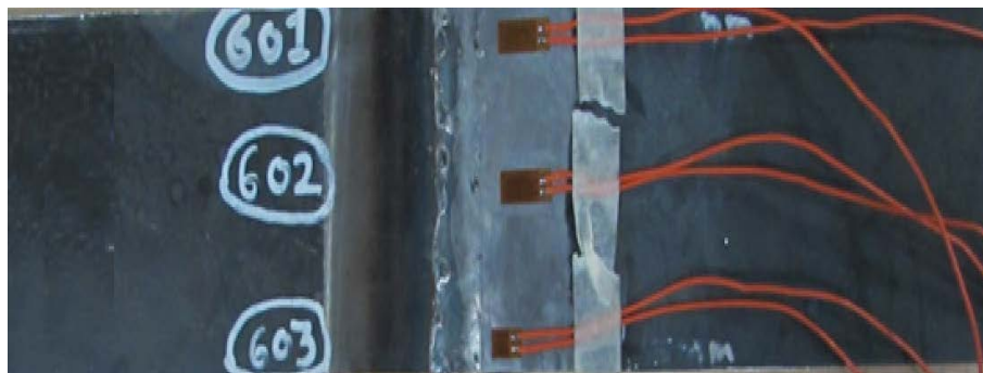
Fig. 4. Strain gauges sample of backing strip weld joint.
