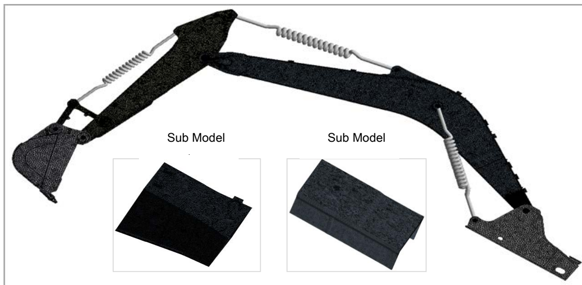
Fig. 21. Mesh model at Assembly level and sub-model level 1 and 2.
