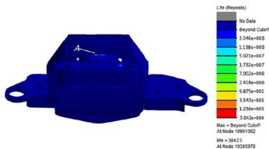
Fig. 11. Fatigue life results of wavelet packet analysis
