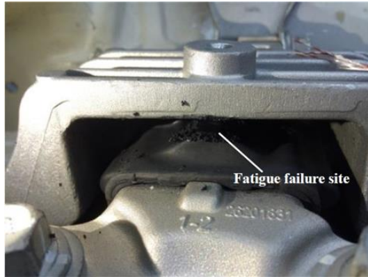
Fig. 13. Fatigue failure site of engine mount
