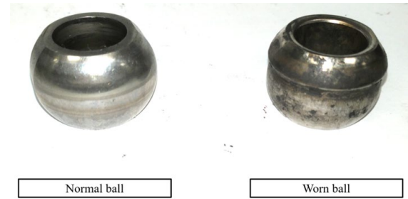
Fig. 4. Comparison of a normal ball with a worn ball.
