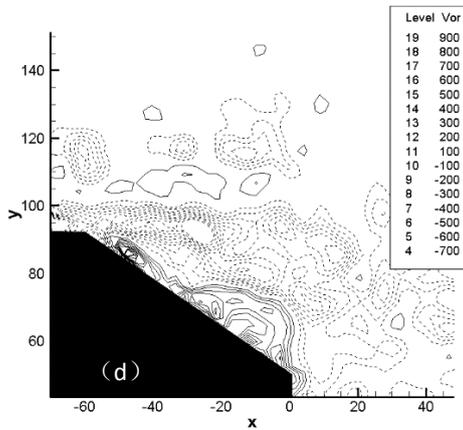
Fig.3. Typical development of the K-H instability from flow visualization(a) (b) (c) and the iso-contours of vorticity level (d) in the  $x-z$  plane at  $y = 0$
