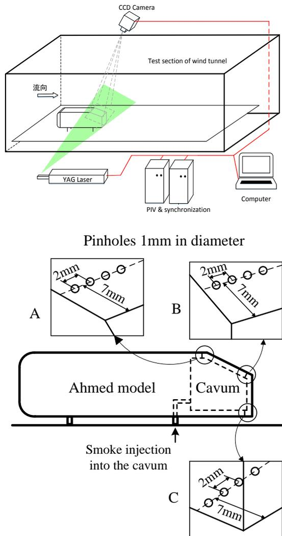
Fig.1. Experiments setup (top) and Ahmed model (under)
