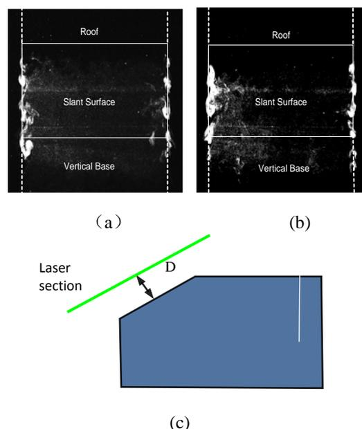
Fig.2. Typical photographs from flow visualization in the plane parallel to the slant surface and the distance is (a)  $D=15$ mm, (b) 20mm, (c) the laser section.
