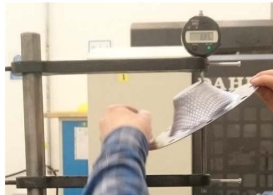
Fig. 11. Measuring of sheet thickness.
