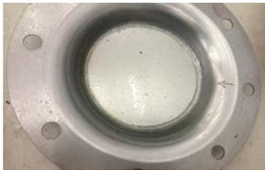
Fig. 5. Failure on 65° formed specimen.
