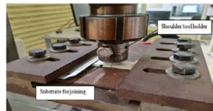
Fig. 3: Welding setup for FSSW on vertical milling machine
