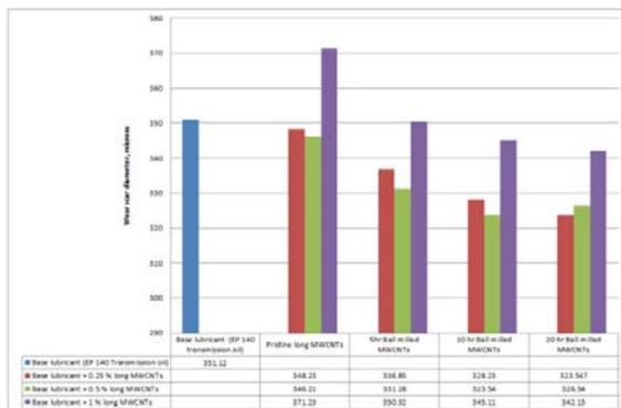
Fig. 6a Variation of wear - scar diameter of test samples
