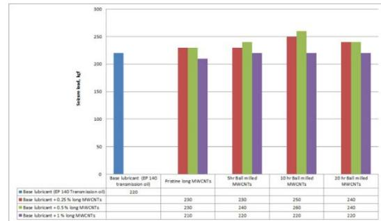
Fig. 6c Variation of seizure load of test samples
