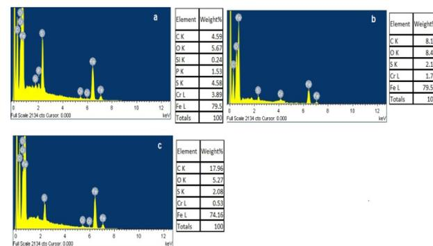
Fig. 9 EDX spectrum of the worn ball a) tested with base lubricant b) examined with lubricant dispersed with 0.25 % ten-hour BM MWCNTs c) tested with lubricant dispersed with 0.5 wt% ten-hour BM MWCNTs
