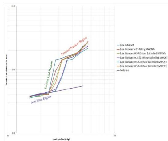
Fig. 8 variation of wear - scar diameter with the applied load during EP test
