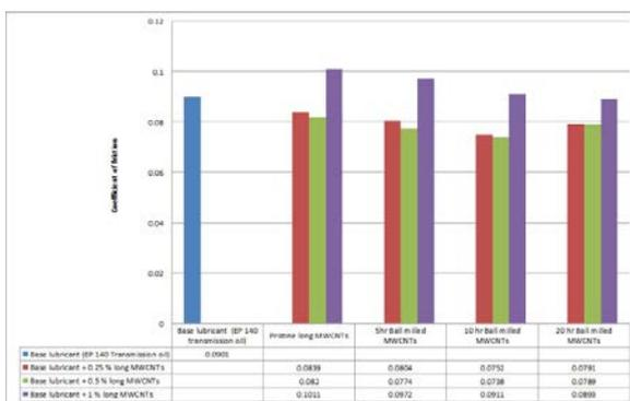
Fig. 6b Variation of friction coefficient of test samples
