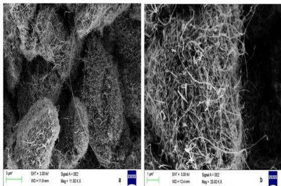
Fig. 1 HRSEM images of a) Pristine MWCNTs b) five hour ball-milled MWCNTs
