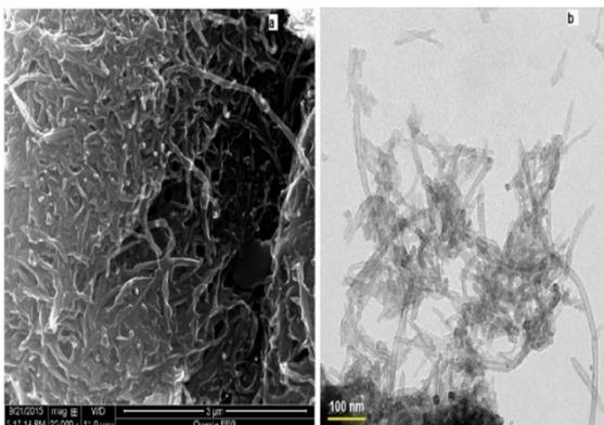
Fig. 2 HRSEM images of a) ten-hour ball-milled MWCNTs b) twenty-hour ball-milled MWCNTs
