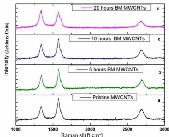
Fig. 3 Raman spectroscopy of MWCNTs a) Pristine MWCNTs b) five hour ball-milled MWCNTs c) ten-hour ball-milled MWCNTs d) ten-hour ball-milled MWCNTs
