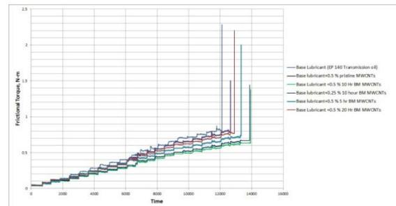
Fig. 7. Variation of friction torque with the time during friction test
