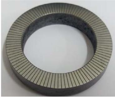
(b) Physical map of groove micro texture friction pairs
