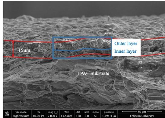
**Figure 2.** The cross-sectional morphologies of MAO coated LA91 alloy.
