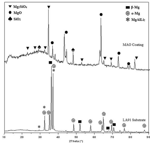
**Figure 3.** The XRD patterns of the LA91 alloy and MAO coating.
