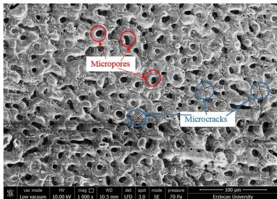
**Figure 1.** The surface morphologies of MAO coated LA91 alloy.
