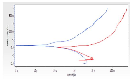
**Figure 4.** The potentiodynamic polarization curves (Red one is LA91 substrates and Blue one is MAO coating).
