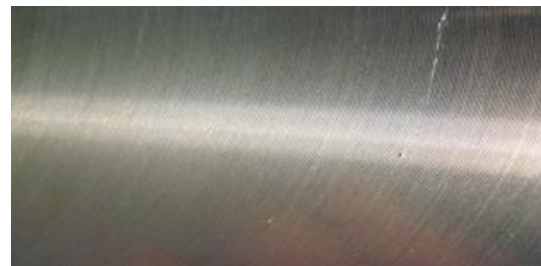
Fig 19 Surface pattern under the conditions of cutting speed of 254.34m/min, feed rate of 200mm/min and axial depth of cut of 1mm
