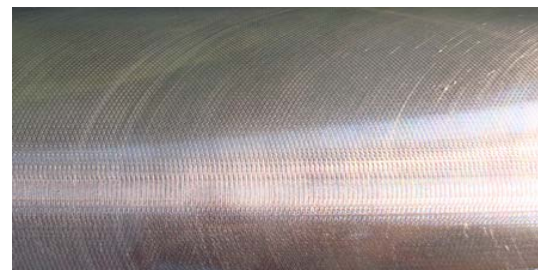
Fig 18 Surface pattern under the conditions of cutting speed of 143.3m/min, feed rate of 400mm/min and axial depth of cut of 0.5mm
