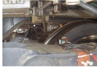
Figure 13. Measurement of acceleration through field test (sensor kept at bogie level).
