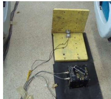
Figure 14. Measurement of acceleration through field test (sensor kept at floor level of central bogie pivot).
