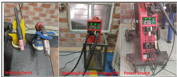
Fig. 3. GTAW Welding Setup.
