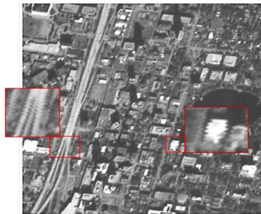
Fig. 1. Example of micro-vibration effect on geometric distortion (Zhang et al. 2011).
