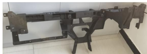
Fig. 11. The manufactured prototype of the CFRP steering column support assembly
