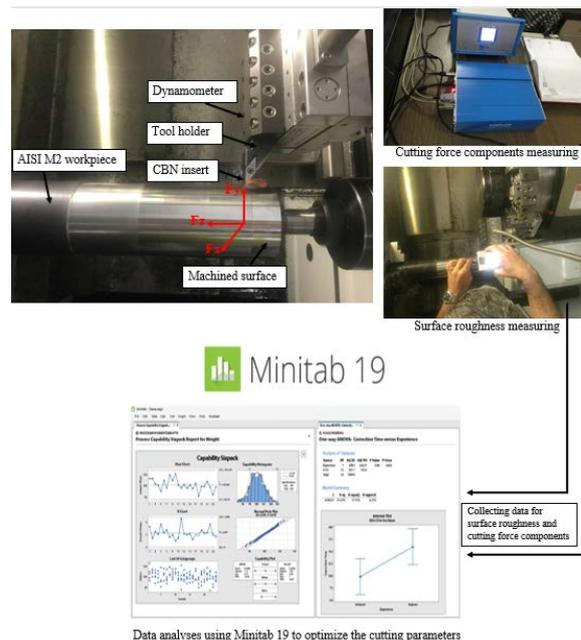
Fig. 3. Experimental setup
