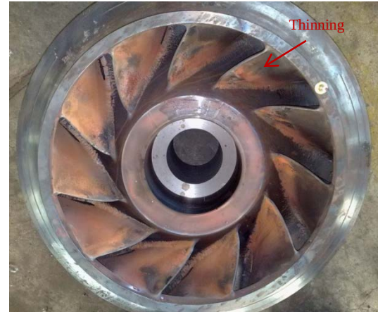
Fig. 1. The local thinning of the blade's leading edge in a shrouded impeller caused by erosion.
