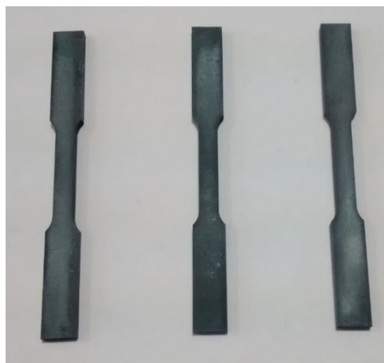
Fig 2. Tensile Samples of ZA-27 hybrid nanocomposites
