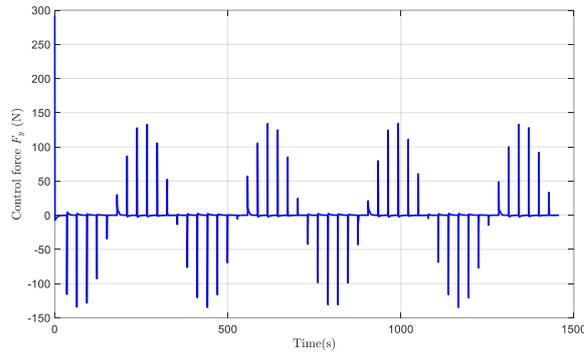
Fig. 26 History of the control force  $F_y$  in Y axis
