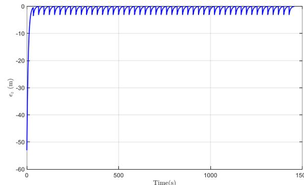
Fig.21 History of tracking error  $e_z$  in Z axis
