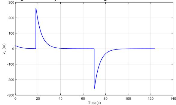
Fig. 4 History of the tracking error  $e_y$  in y axis
