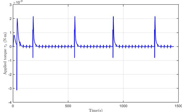
Fig. 28 History of the applied control torque  $\tau_\phi$
