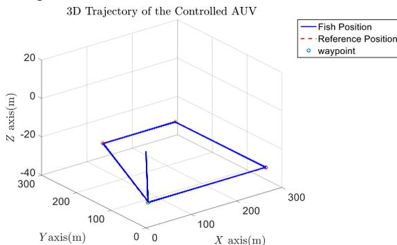
Fig. 2. Trajectory of the guided AUV for Case 1
