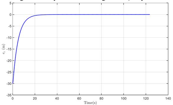
Fig. 5 History of the tracking error  $e_z$  in z axis
