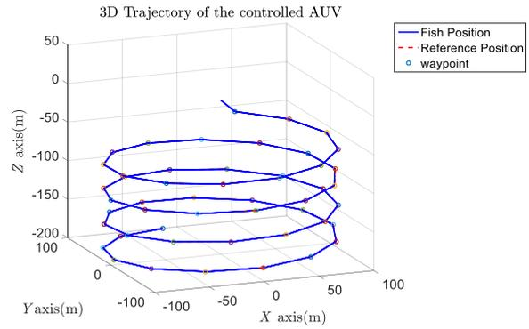
Fig. 18 Trajectory of the guided AUV for Case 2
