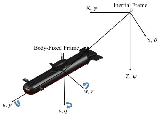
Fig. 1. The AUV geometry illustration
